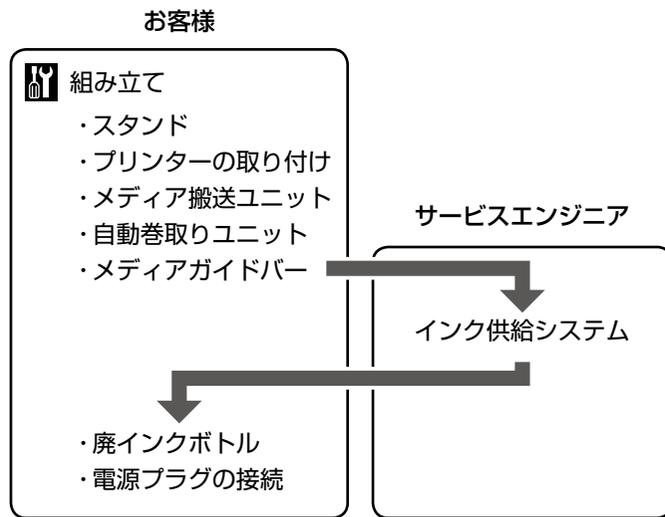
Contact a service engineer to attach the "Ink Supply System". Attempting to perform these tasks yourself could result in product malfunction or damage to the product and will void the product warranty.
