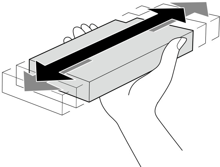
To maintain optimum printing conditions, before installing the white ink cartridge in the printer, shake it quickly back and forth as shown in the illustration in roughly five centimeter movements, about 100 times within about 30 seconds. After installing the white ink cartridge in the printer, remove and shake it over 10 times once a week.
